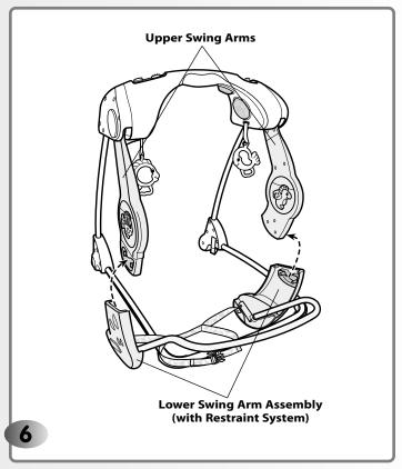
• Fit the lower swing arm assembly to the outer side of the upper swing arms.
